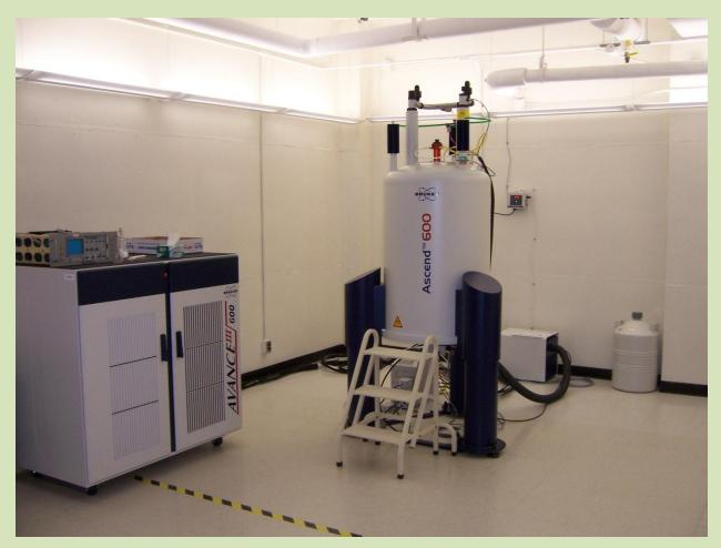
A new Bruker Avance III 600 MHz NMR spectrometer has recently been installed at Binghamton University. This instrument will serve as the cornerstone of a **Regional NMR Facility**, which is being established to provide regional colleges and universities with the means to perform liquid and solid state NMR experiments, which their own instruments were not designed to run.
