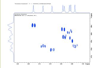
After linear prediction of 4096 complex data points in the <sup>13</sup>C dimension the peak separation in the <sup>13</sup>C projection is adequate to provide a low-resolution <sup>13</sup>C spectrum:
